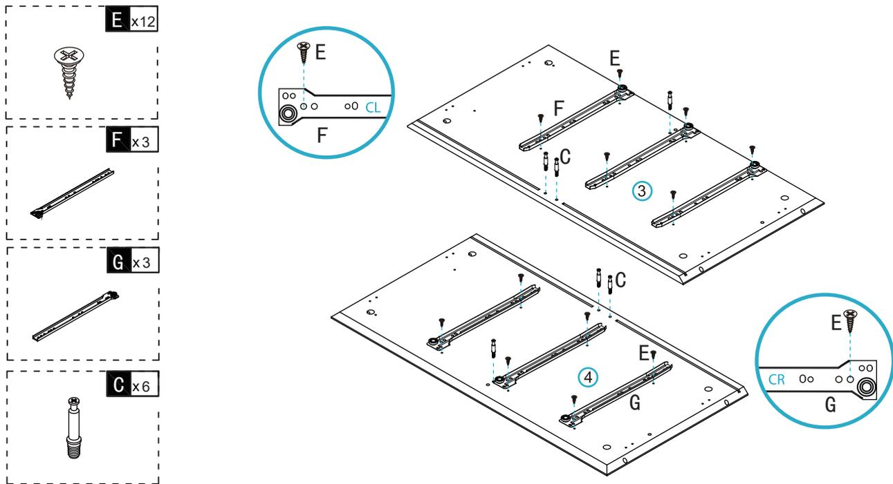
**EN** Please find the exact hole for installation, otherwise it will be misaligned. The screws on the drawer slide must be leveled, otherwise it will affect the smoothness of the drawer.
