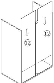
Insert back board 12 along grooves as shown.
