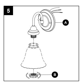
Install light bulb (not included). Use 60-watt max. standard-base incandescent bulb or halogen/ CFL/LED equivalent.
