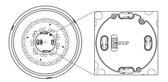
This fixture allows the user to set the desired CCT color temperature from a soft white (2700K), to a cool white (4000K) or a daylight white (5000K) output. This allows the light from this fixture to match the CCT of other lights within the same room or to set the desired ambient room lighting.
