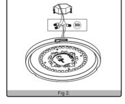
3. Lift fixture pan (A) up toward ceiling and carefully tuck wires into outlet box. Align keyholes on fixture pan (A) with screws (aa), then twist fixture pan (A) until the screws (aa) engage the narrow end of the keyhole slots. Tighten the screws (aa) to secure the fixture.
