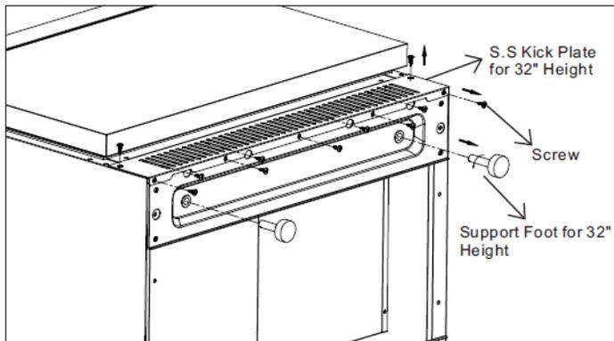
5. Reusing the original screws, install the kick plate and supporting feet for 34.25" height,
