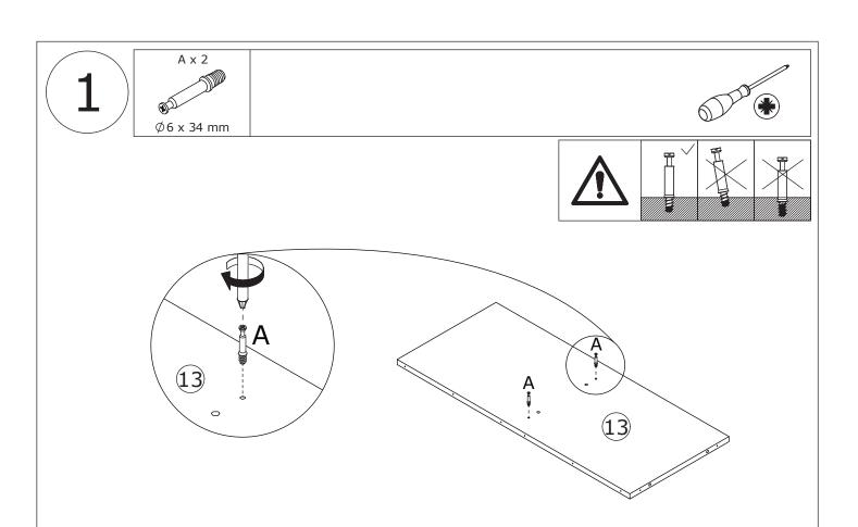
Screw eccentric rod(A) into board 13 with a screwdriver.
