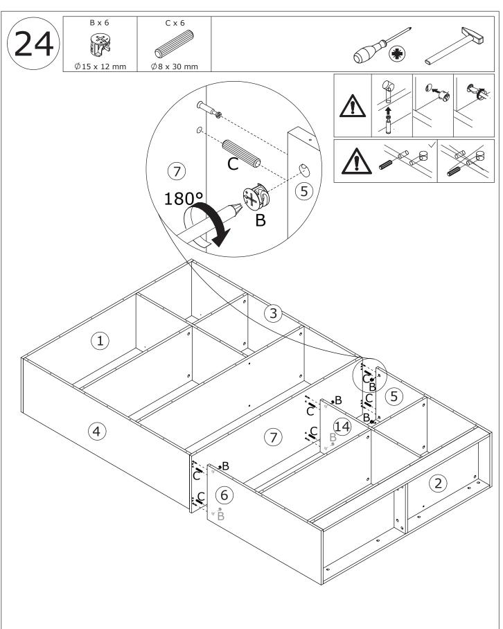
Connect the two assembled components using wooden dowel(C), add cam lock(B) and turn clockwise to tighten as shown.
