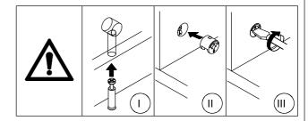
Turn cam locks clockwise to tighten.
