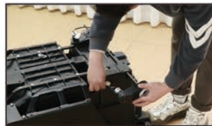
3. Double headed wire on the L side of the car body, single wire on the R side. Continue the power cord into the car body and install the motor on the other side. The installation method of the motor is the same
