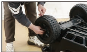
4. Align the motor flower groove and thread the rear wheel onto the rear axle. Insert the gasket and tighten the nut. The installation method for the rear wheel is the same. Use the installation tool to tighten the nuts on both sides of the rear wheel at the same time
