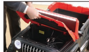
18. Connect the power cord on the windshield and align it Install the front cover of the card slot and fasten the locking buckle
