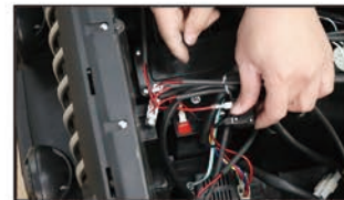
15. Remove the white insulation cap and connect the battery to the battery Source line, test power supply
