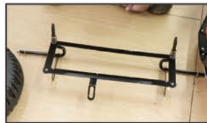
6. Cut open the tape and remove the steering shaft plate, align the steering front axle, unscrew the two nuts on the shaft end, take out the shock absorber spring, put on the steering shaft plate, and install the shock absorber spring
