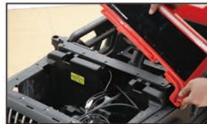
17. Unscrew the four screws reserved for fixing the windshield panel Thread the power cord into the vehicle and align it with the card Install the windshield in the slot and tighten the screws
