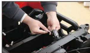
16. The letters on the steering wheel face downwards, connecting Steering wheel power cord, remove excess power Insert the wire into the vehicle and install the steering wheel
