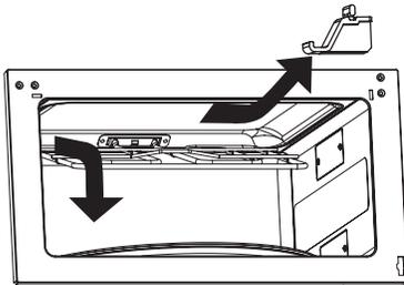
2. Lower the front of the broil element to access the ceiling for cleaning.
