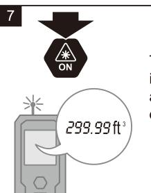
The result is shown in the main line and the measured distance above.
