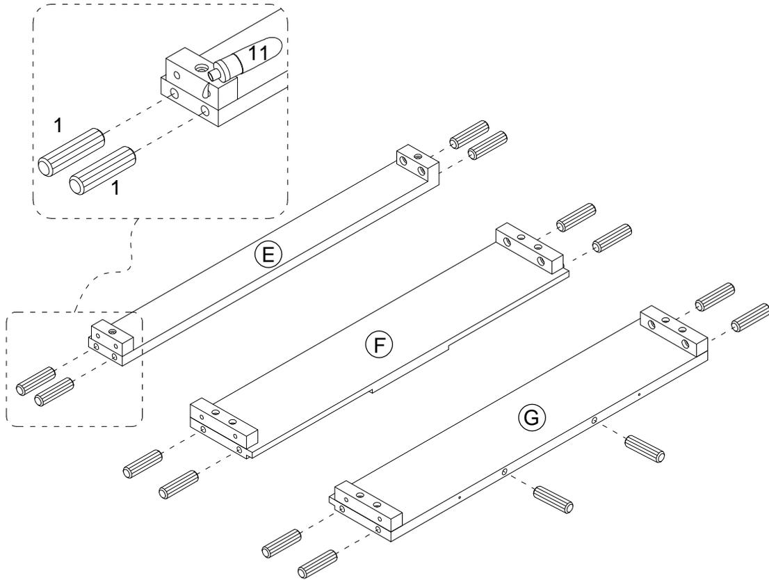
Glue the wood dowels 1 into the inner holes on the front upper rail E ,F and G .
