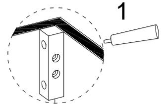
To install the Top (1) to the vanity (2). Apply silicone caulk to the top edge of the wood cabinet. With the help of another adult, gently lower the Sink top with assembled sink onto the cabinet. Make sure the Sink top is flush with the back side of the wood cabinet and the wood cabinet left and right side walls.
