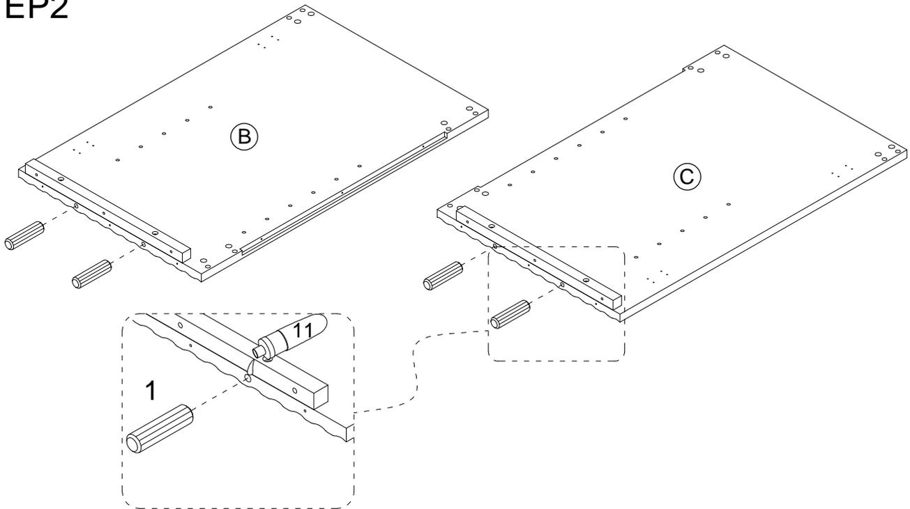
Glue the wood dowels 1 into the inner holes on the front upper rail Band C .
