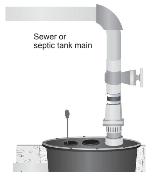
**4** Attach a 2-in male adapter to the vent opening on the top of the lid. Using 2-in. PVC and a 2-step PVC glue system, connect the vent opening to the sewer vent system. Use pipe tape to seal this connection. A union is recommended for easy pump service.
