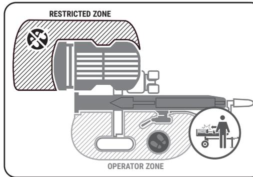
Always keep bystanders away at least 10 feet (3m) from this machine. Only one person should operate the log splitter and load the logs.
