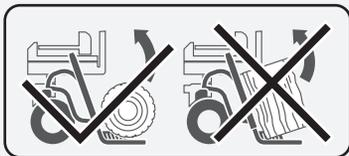
3. Give the control lever a backward thrust, wait until the wedge starts to move, release the control lever, and then the log lift table attachment starts to rise. (See **Figure 27b.**)
