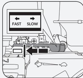
6. Pull the recoil starter until engine compression has become difficult to pull. Let the recoil return to the home position, then pull quickly to start the engine. Repeat steps as needed. Fully open the choke and set the throttle to the FAST position, before operating the unit.
