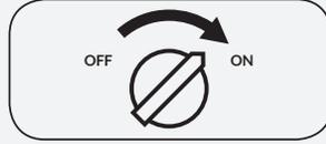
2. Move the engine switch to the ON position.
