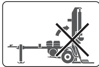
Vertical operating position is prohibited when the log lift table attachment is attached.
