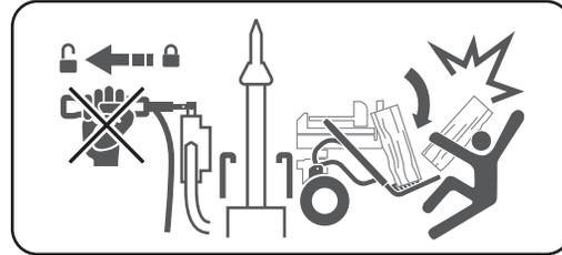
When the wedge is extended and not fully return back, do not pull the control lever outwards, otherwise the log lift table attachment may suddenly drop down, risks of falling the log, damage and injury.
