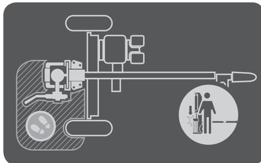
**WARNING** Vertical operating position is prohibited when the log lift table attachment is attached.
