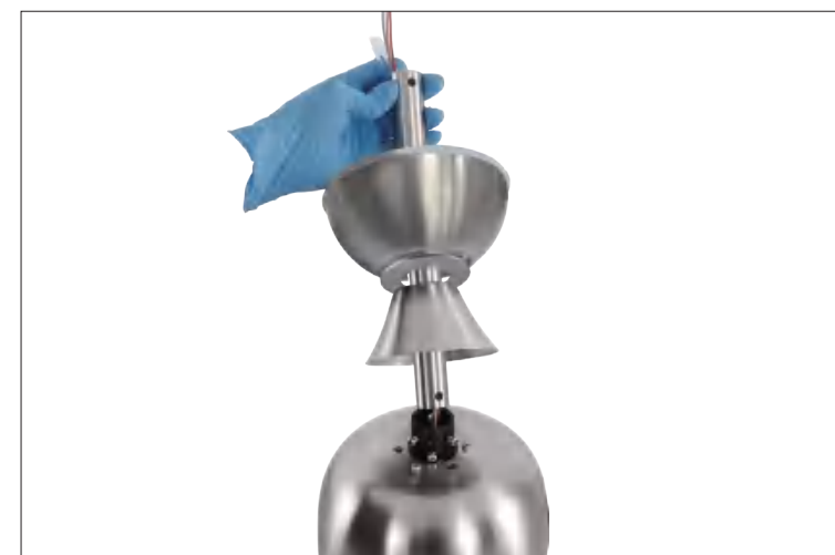
Step 6 Pull out the R-pin from the rod.
