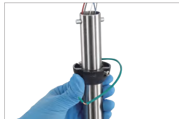
Step 8 Push the hemisphere up, Align the small rod with the notch on the hemisphere.
