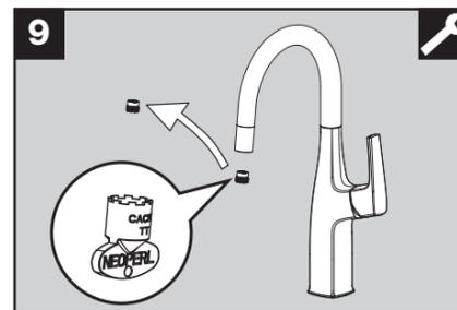
Remove aerator using the aerator key (12).
