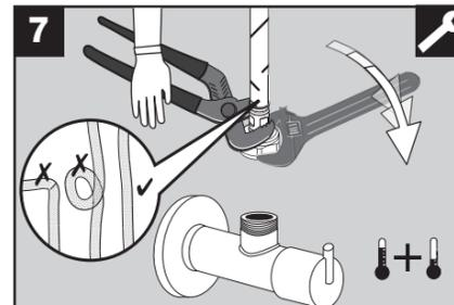
Connect hot supply line (red) and cold supply line (blue) to hot and cold water valves.
