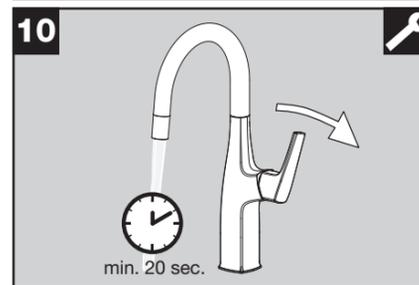
Turn the faucet on and let the water run for at least 20 seconds to ensure the lines and the faucet are flushed.
