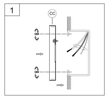
1. Attach the round mounting plate (CC) to the outlet box using the mounting screws supplied with the outlet box (not provided). Tighten securely.
