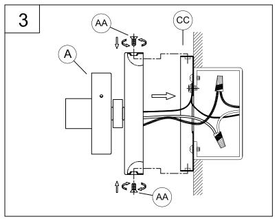
3. Attach the fixture (A) to the round mounting plate (CC), aligning the holes in the fixture (A) and the holes of the round mounting plate (CC). Using the two flat screws (AA), tighten the fixture (A) against the mounting surface.
