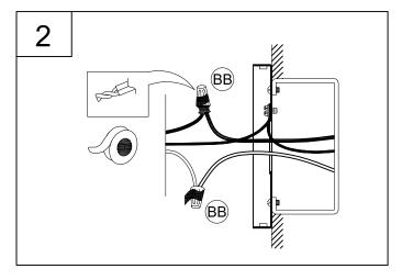
2. Strip 3/8" of insulation from the electrical wire ends. Using wire connector (BB), connect the WHITE fixture wire to the WHITE supply wire from the outlet box; connect the BLACK fixture wire to the BLACK supply wire from the outlet box.
