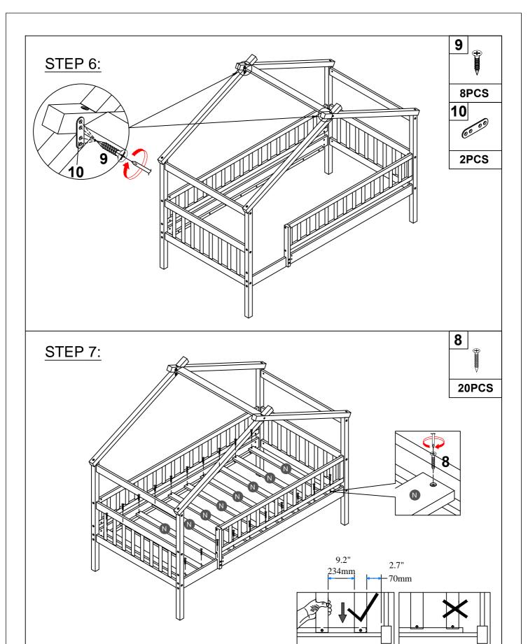
Note: Do not lock the screws of the bed slats to the outermost edge of the bed slats, you need to leave a certain space at the edges, otherwise it will cause the board to break. Do not lock the bed slats on the edge of the wood, please hold firmly before screwing, hold it in place with one hand, then lock the screw.
