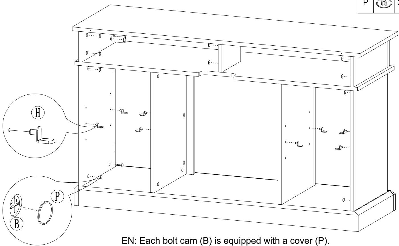
EN: Each bolt cam (B) is equipped with a cover (P).
