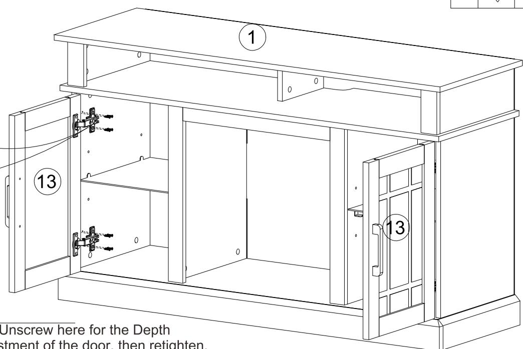
**EN:** Unscrew here for the Depth adjustment of the door, then retighten.
