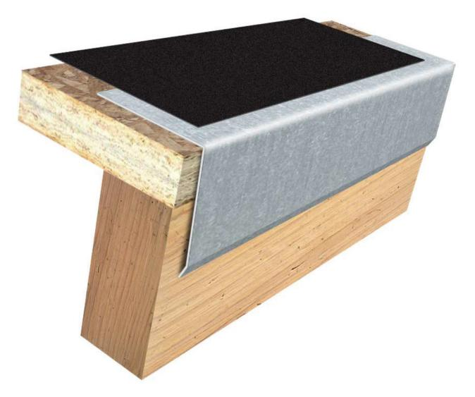
Begin installation along the eaves, starting at a corner and working your way around, overlapping each succeeding piece of drip edge by 2-3 inches.
