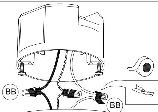
3. Strip 3/8" of insulation from the electrical wire ends. Using wire nuts (BB), connect the WHITE fixture wire to the WHITE supply wire from the junction box; connect the BLACK fixture wire to the BLACK supply wire from the junction box.
