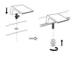
3. Screw spout fixing parts to spout, unscrew the washers and the fixing nut, place spout to bathtub hole, reinstall washers and fixing nut then hand tighten them.
