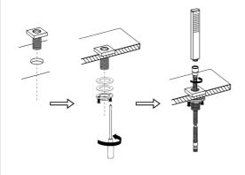
6.Unscrew the washers and fixing nut from cover & connector, place cover & connector to bathtub hole, reinstall the washers and fixing nut; connect hand shower and shower hose then place the shower hose to the bathtub hole as picture show.
