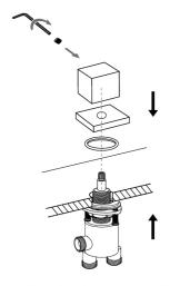
5. Pass the diverter valve part through bathtub hole as picture shows, reinstall the rubber washer, knob & cover then tighten the diverter fixing parts and the screw in the knob.
