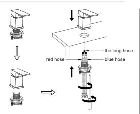
2.Disconnect handle fixing parts from handle parts, put red & blue hoses and the long hose through thread pipe and connect them to the handle part as picture shows, screw thread pipe to handle part then tighten the handle fixing parts.
