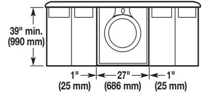
For closet installation, with a door, the minimum ventilation openings in the top and bottom of the door are required. Louvered doors with equivalent air ventilation openings are acceptable.
