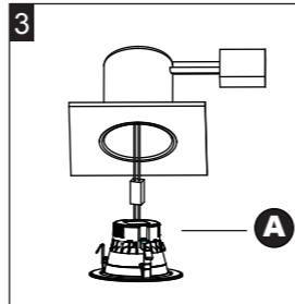
4. Carefully route wires into fixture. Push retrofit into recessed housing until the trim is flush with the ceiling surface.
