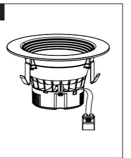
2. Screw adapter (B) into socket in recessed housing.
