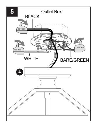
Wrap electrical tape (not included) around each individual lever wire connector down to the wire
