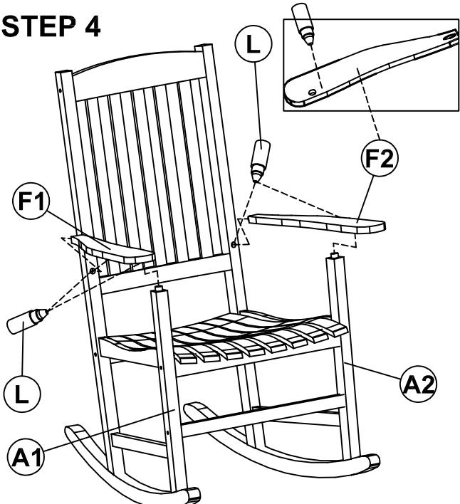
Upright the chair. Apply glue (L) to all holes in arms (F1&F2) and side frame (A1&A2), As shown. Next, attach right arm (F1) and Left arm (F2) in side frame holes and tenons, as shown.
