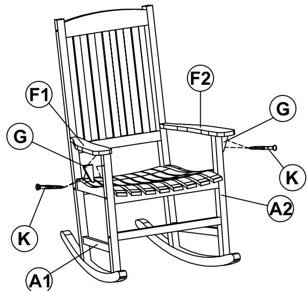
Attached Support (G) to right and left side frame (A1 & A2), secure using 1 1/4" screws (K) as shown.
