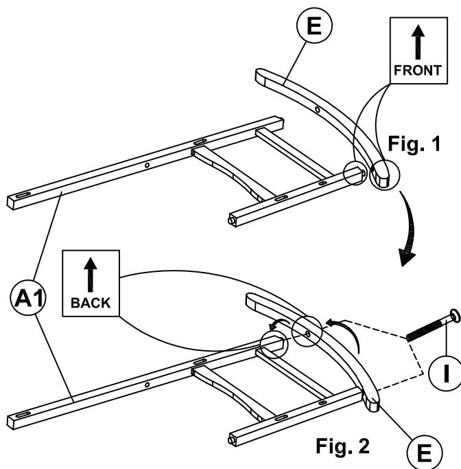
Attached each rocker (E) to right and left side frame (A1 & A2) as picture shown, connecting front of rocker to front legs first then the back of rockers. Secure connections with 1 3/4" Bolts (I).
