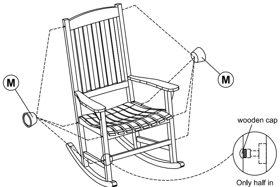
Make sure all parts are connected and tighten all bolts and screws completely using screwdriver. Tap in the wooden caps (M) to cover bolts head using rubber mallet.
