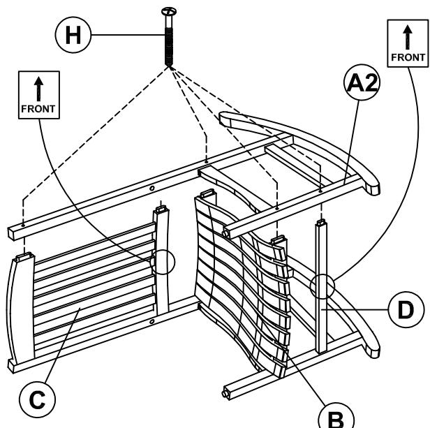
Install Seat (B), back support (C), and Apron (D) into corresponding holes of right side frame (A1). Attach the left side frame (A2) onto seat (B), back support (C), and apron (D). Secure left side frame (A2) using 1 1/4" bolts (H), as shown.
