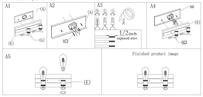
Step A1: Unscrew the ball knobs (G) from back plate(E) then gently remove mounting plate (A)
