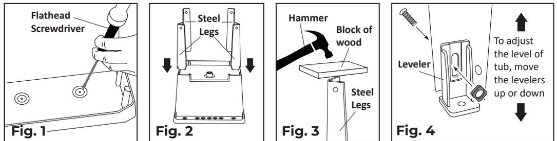
1. Place the laundry tub on a clean surface, such as a blanket or cardboard, and turn the tub upside down to allow for the removal of the pre-formed knockouts. These will accommodate the faucet that is going to be installed. The hole plugs may be removed by a flathead screwdriver or a small chisel and a hammer (see Fig. 1).
