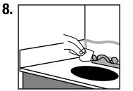
With a caulk edging tool, run it across the seams to clear away excess silicone & caulk (this technique will leave a clean line of silicone & caulk over the seams).
