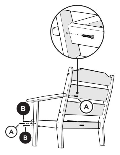
Partially thread each screw into pilot holes by hand before fully tightening.
