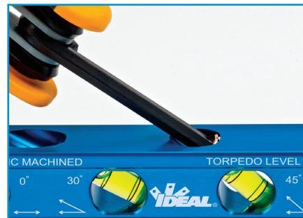
4. Reinstall O-ring and set screw
