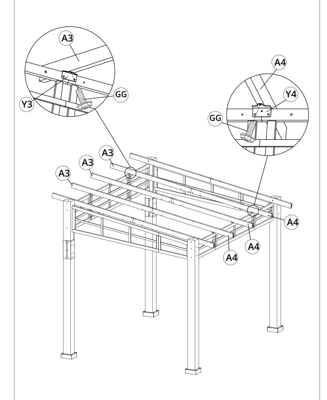
Note: A3 A4 parts do not need to be locked tightly for subsequent installation
