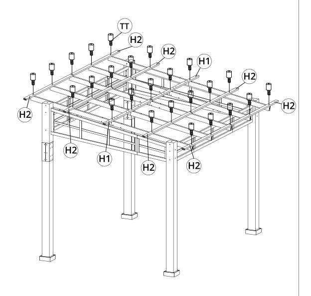
Note: H1 H2 parts do need to be locked tightly for subsequent installation
