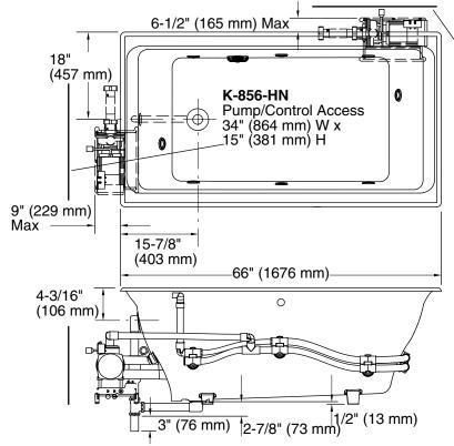
No change in measurements if connected with drain illustrated. (K-7147-AF or K-7147M-AF)
