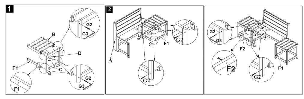
Step 1: attach the seat (B) to the side (C), joint bar (D), front bar (F1) as shown on the picture. Then use the Allen screw (G2) to tighten together these parts.
