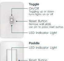
Remove wall plate, use pin to press reset button
