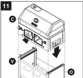
12. Secure lid and firebox assembly (C) on top of left cart assembly (V) and right cart assembly (O) using four M6x20 bolts (BB).
