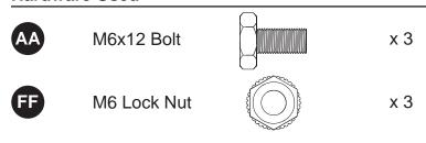
21. Attach lid handle assembly (D) to lid and firebox assembly (C) using two M6x12 bolts (AA).
