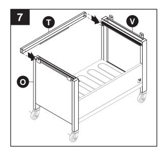
8. Secure upper door brace (T) using four M6x12 bolts (AA).
