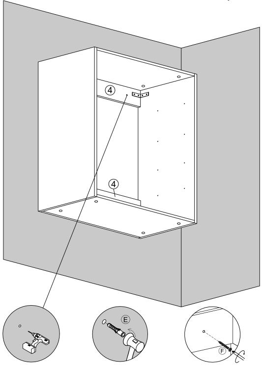
DETAIL HOLE FOR WALL FIXING Note: hammer is not included.
