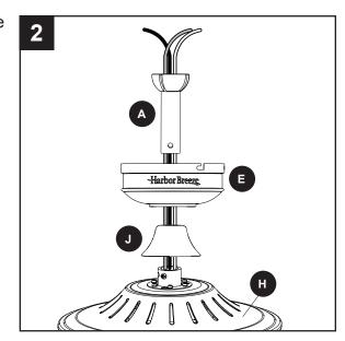
3. Slide the downrod (A) into the yoke of the motor assembly (H), align the holes, then re-install the downrod pin (B) and downrod clip (C). Secure with set the two screws (Q) and slide the yoke cover (J) down until it rests on top of the motor assembly (H).
