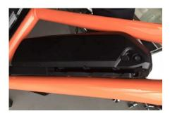
Important: The battery must be locked when riding or it may fall out. The key does not have to be in to operate the bike.
