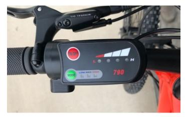
**Note**: Before mounting the bike to ride, hold the brake lever. It cuts off the main power to the bike. It is always safest to mount the bike before turning on the bike, as turning it on enables the throttle. If you
