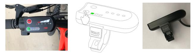
You can set Pedal Assist through 3 speed modes Low, Mid and High. Low is the slowest and High is the fastest.
