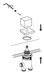
5. Pass the diverter valve part through bathtub hole as picture shows, reinstall the rubber washer, knob & cover then tighten the diverter fixing parts and the screw in the knob.
