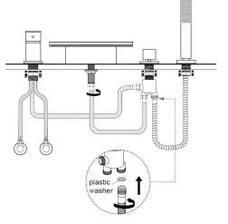
7.Connect the red & blue hose to the hot and cold angle valves, connect the long hose to the hole on the side of diverter valve part, connect the short hose to the spout and the left hole of the diverter valve part, put the plastic washer on the connector of shower hose then screw it to the right hole of diverter valve part.
