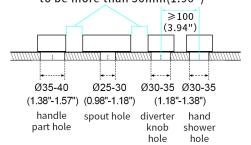
1.Drill holes as recommended openning holes size (Note: holes distance should as picture shows).
