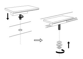
3. Screw spout fixing parts to spout, unscrew the washers and the fixing nut, place spout to bathtub hole, reinstall washers and fixing nut then hand tighten them.
