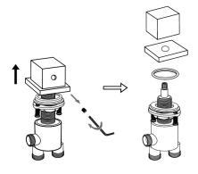
4.Use allen key to loose the screw in knob then disconnect knob & cover, rubber washer, diverter valve part as picture shows.
