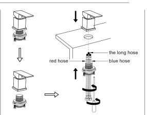
2.Disconnect handle fixing parts from handle parts, put red & blue hoses and the long hose through thread pipe and connect them to the handle part as picture shows, screw thread pipe to handle part then tighten the handle fixing parts.
