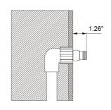
16. Drill out the two marks and secure the mounting adapters to the finish wall.
