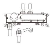
3. After the wall is finished, remove the plastergaurd from the valve body and cut the valve body casingflush with the wall if necessary. Discard the platergaurd.
