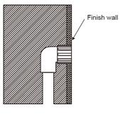
21. Wrap the threads of the shower head arm with teflon tape and screw it into the wall connection as shown in the images.
