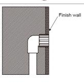
14. After verifying the center of the water outlet and distance needed for the mounting adapters mark the locations ensuring that both marks are level.
