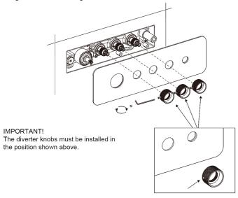
7. Screw the push button caps on until the O-ring is no longer visible, making sure that they are even with the end of the knobs.
