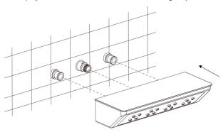
18. Tighten the two M5 screws to secure the back spray head.
