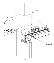
2. Wrap teflon tape around the threads of the male adapters and connect the hot, cold, shower head, and back spray head water lines to the valve body.
