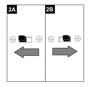
2C. **IMPORTANT:** Reverse switch must be set either *completely* to the LEFT or *completely* to the RIGHT for fan to function. If the reverse switch is set in the middle position, fan will not operate.
