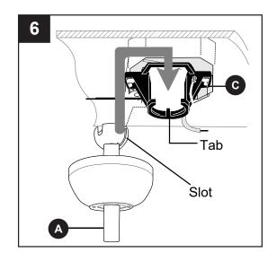
6. Install ball end of downrod (A) into opening of mounting bracket (C). Align slot in ball with tab in mounting bracket (C).
