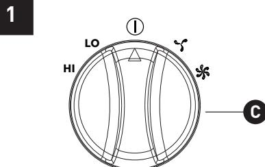
2. Select a heat or fan setting by turning the MODE dial on the control panel (C) to the LO, HI, fan speed 1 or fan speed 2 position.
