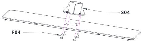
/Place the pedestal pole (S02) into the pole support. Align the three inner holes and fix together using three M8x1in (25mm) screws (F04). Fully tighten.
