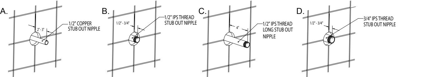
**Fig. A. 1/2" Copper Pipe Slip Connection**
