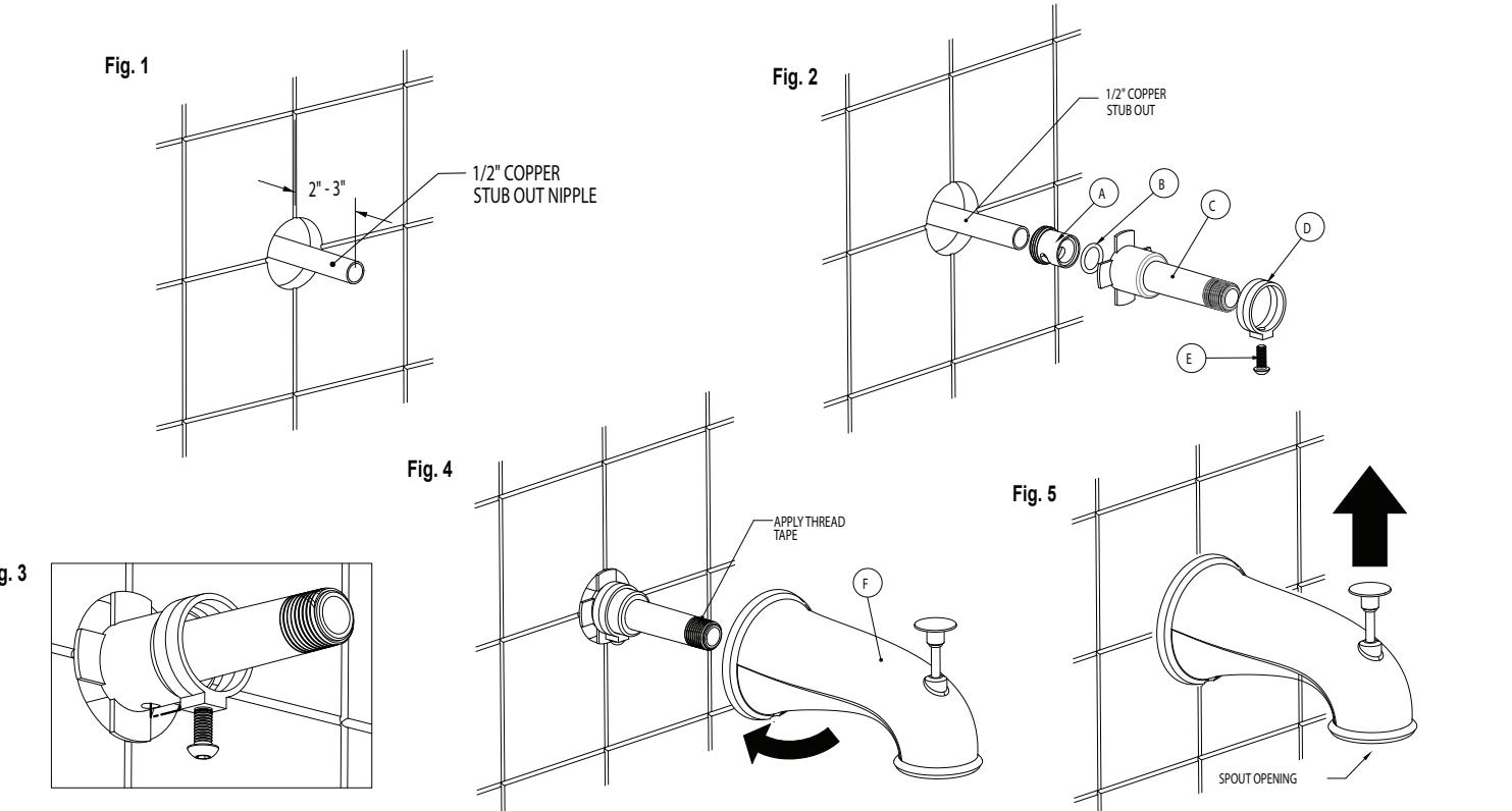
**Fig. B. 1/2" Male Threaded Connection with Short Stub Out Connection**
