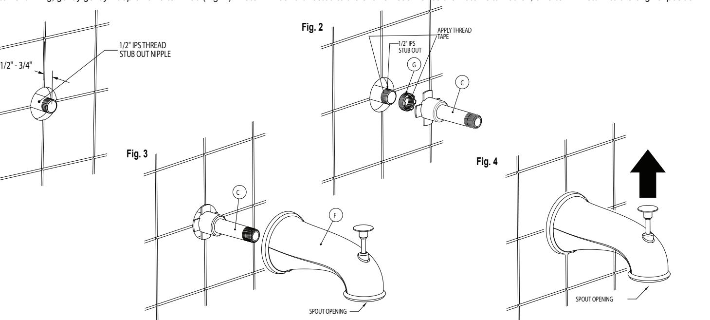
**Fig. C. 1/2" Male Threaded Connection with Long Stub Out Nipple**
