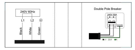
Black live wire L1, white live wire L2, green ground wire. The whole machine cannot be powered on if any of the black and white wires are not contacted well.
