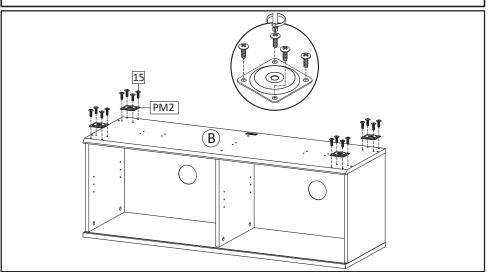
**STEP4**: Install Mounting Plate (PM2) and secure with screw M 4.5 x 12.5 mm (HW15) on Bottom Board.
