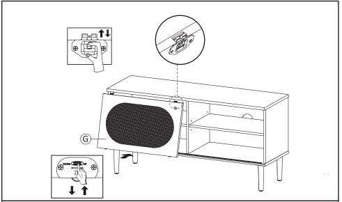
**Step10**: Slide in the door and insert the Sliding Top (HW8) pin into the groove of Top Board. Position the Sliding Bottom (HW9) into the grooved sliding track. Adjust gap of the door by scrolling the button on Sliding Roller (HW9). Follow the down and up direction. Slide the door to the right and left, ensuring the door has been placed properly in the provided track.
