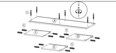
**STEP1**: Insert Cambolt (HW1)into Top Board (A). Insert Dowel (HW4) into Side Board Left (C), Side Board Right (D) and Center Board (E).
