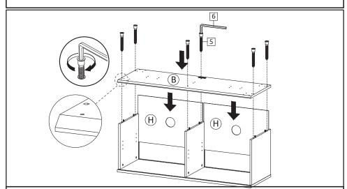
**Step3**: Insert Back Boards (H) as figure. Put Bottom Board (B) and secure with Screw M7x50 mm (HW5), tighten screws using Allen Key (HW6).
