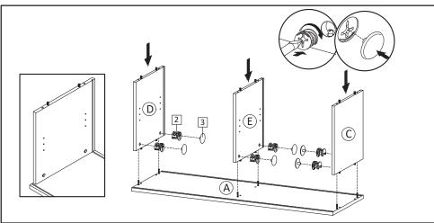
**STEP2**: Attach Side Board Left (C), Side Board Right (D) and Center Board (E),into Top Board (A). Insert Camlock (HW2) then tighten using screwdriver. Put Screw Cap (HW3) over the camlock.
