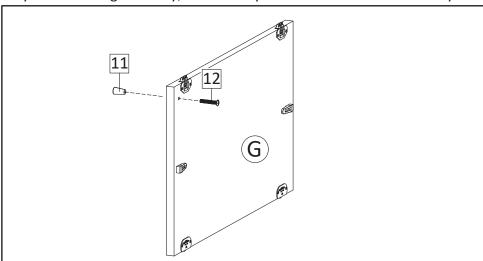
**STEP9**: Insert Handle (HW11) and Screw M4x25 mm (HW12) into Door.
