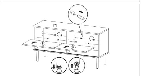
**STEP7**: Insert Shelf Pin (HW7) in between Side boards and Center board on the desired level. Then place the Adjustable Shelf (F) onto the Shelf Pin. Place your furniture on level floor. The legs come with adjustable leveler, adjust it as needed until your furniture stands steadily on the floor.
