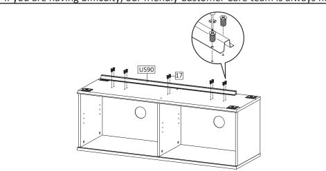
**STEP5**: Place Anti Deflection Metal Bar (HW US90), secure with screw M6x12.5 mm (HW17) tighten using screwdriver.
