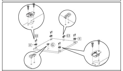
**STEP8**: Insert Sliding Top (HW8) and Sliding Bottom (HW9) using Screw M3.5x13mm (HW10) into Door (G). Tighten with a screwdriver. Install Stopper (HW13).
