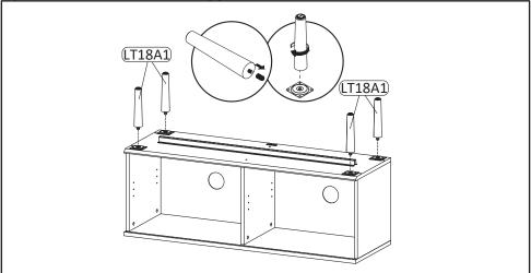
$\mbox{\bf STEP6}:$  Insert Leg (LT18A1) into Mounting Plate, tighten by rotating . the leg clockwise.
