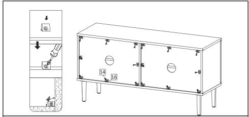
**STEP11**: Use Wedge (HW16), Screw M3.5x15.5 mm (HW14) to tighten the back of media stand by using screwdriver. Align the top board and bottom board in  $90^{\circ}$  position against the side board, before securing the wedges (HW16).
