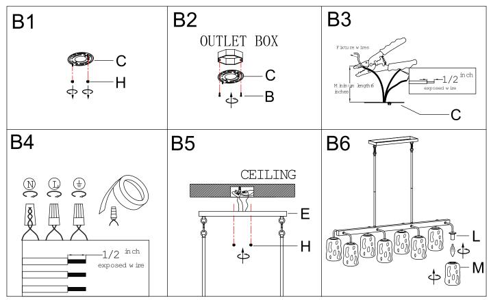
$\label{eq:StepB1} \textit{Step B1} \ \textit{\textbf{w}} \ \ \text{Unscrew ball nuts (H) from mounting plate (C)}.$
