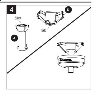
Insert the receiver from remote pack (Q) into the mounting bracket (D) with antenna end first and flat side facing up. Note: The receiver rests directly on the downrod (A).
