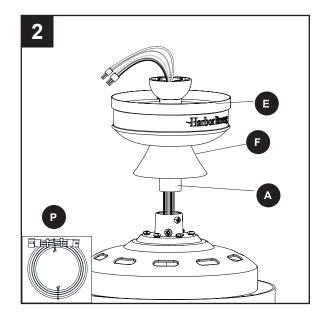
Slide the downrod (A) into the yoke, align the holes, then re-install the downrod pin (B) and downrod clip (C). Secure with set screws (I) and slide the yoke cover (F) down until it rests on top of the motor assembly (H).
