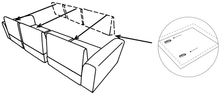
**STEP 5** 1. Use Metal screws① to link Console Back(C) to Console Body (D)
