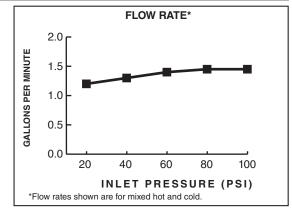
1.5 gpm/5.7 L/min. FLOW RATE
